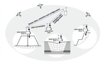
The graphic illustrates the GNSS meter's operation. Rovers collect satellite data and receive RTK corrections from a base station via LoRa, which enables precise positioning. The GNSS meter then transmits sensor data and performance statistics to the gateway using LoRa. Remote configuration is also possible via CMT through the gateway, ensuring flexibility and control.
